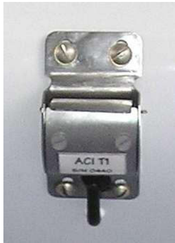
Fig.1- Stall speed vane on the left wing
